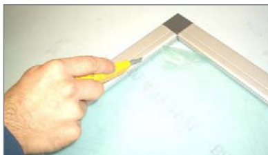
Fig. 2: before silencing, the protective film is removed from the corners of the frame.
