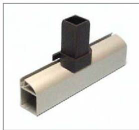
Fig. 13: after machining the seat on the profile, the joint can be secured using two 3.9x19 mm self-threading screws.
